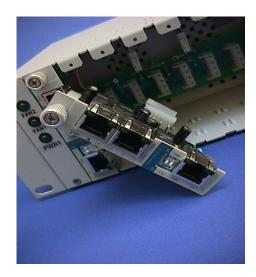
ERMTT1008 plugs into ERM21C, 21 Slot Chassis
